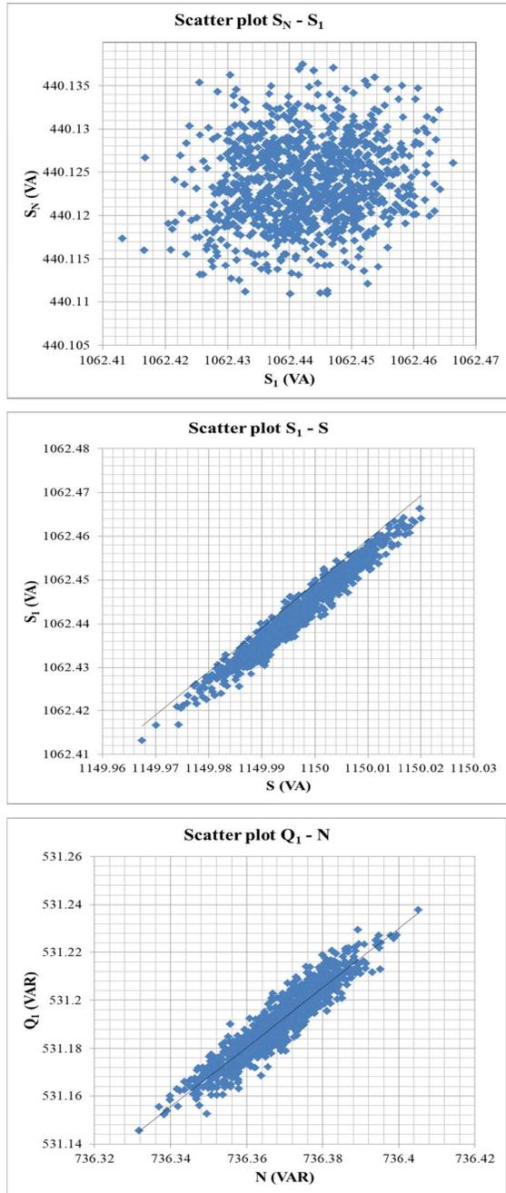
Fig. 2. Results of correlation analysis. Scatter plots of powers pairs ( $S_N$ - $S_1$ ,  $S_1$ - $S$ , and  $Q_1$ - $N$ ). Experimental test with fifth harmonic on both voltage and current;  $30^\circ$  phase shift between both fundamental and harmonic components.
